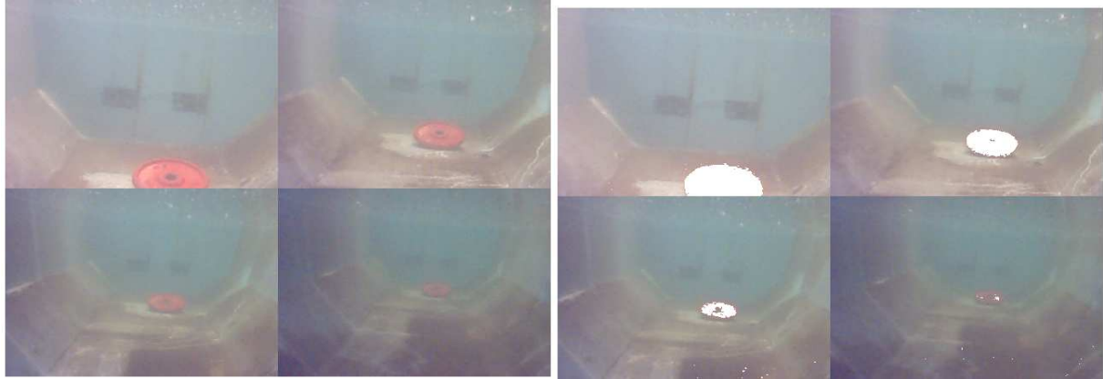
Figure 8: Underwater object detection based on color detection taking color fading into consideration
